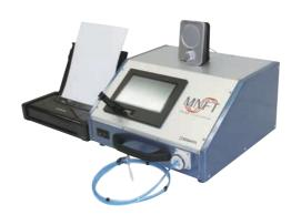
MNFT ver.2 gives the idea to understand the difference whether it is sealed or not. Leakage and pressure inside the mask is detected and visualised at the
